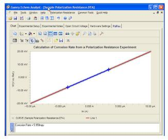
A Polarization Resistance Experiment tDisplayed in the EchemAnalyst. The dhe dark blue curve segment is used to calculate the corrosion rate. Note the Corrosion Rate on the lower portion of the display. More detail is available on the PolRes tab.
