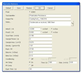
**Setup Window for Polarization Resistance**. Every parameter required to make the Polarization Resistance measurement is available on the single Setup Window. Click **Save** to archive an experimental setup for easy **Restore** later.
