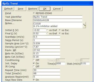
Setup Window for Rp/Ec Trend. Setup Window for Rp/Ec Trend. An Rp/Ec Trend setup is identical to Polarization Resistance for the electrochemical parameters. The Total Time of the experiment is entered along with the repeat time of the Rp measurements. The Analysis Region is the voltage range around Eoc where the slope of the curve is measured. The Base Filename is the file name used to save the multiple data sets in an incremental format.
