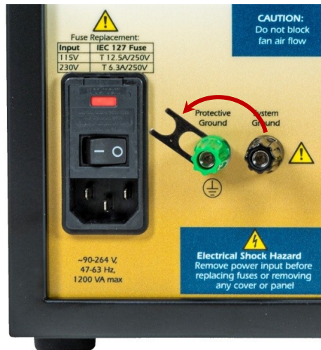
Figure B-4 Storing Ground Jumper When Disconnected
