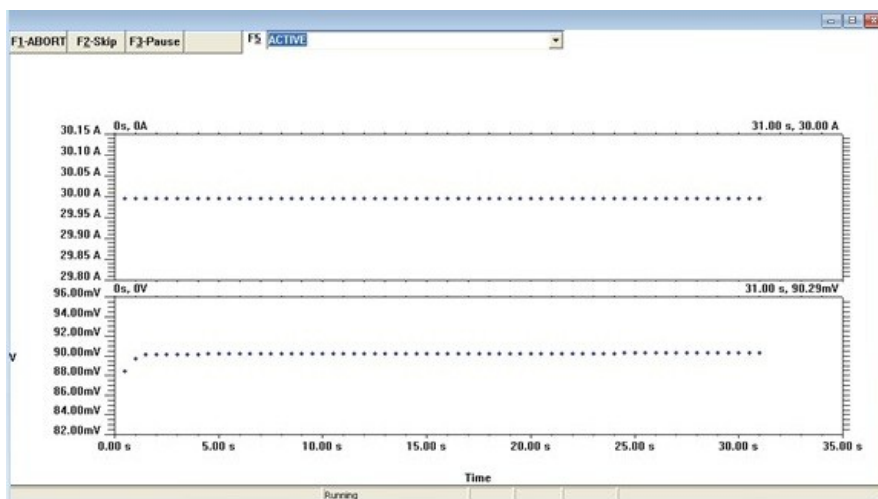
Figure 3-6 Current-versus-Time Curve for 30 A Applied to the Test Cell
