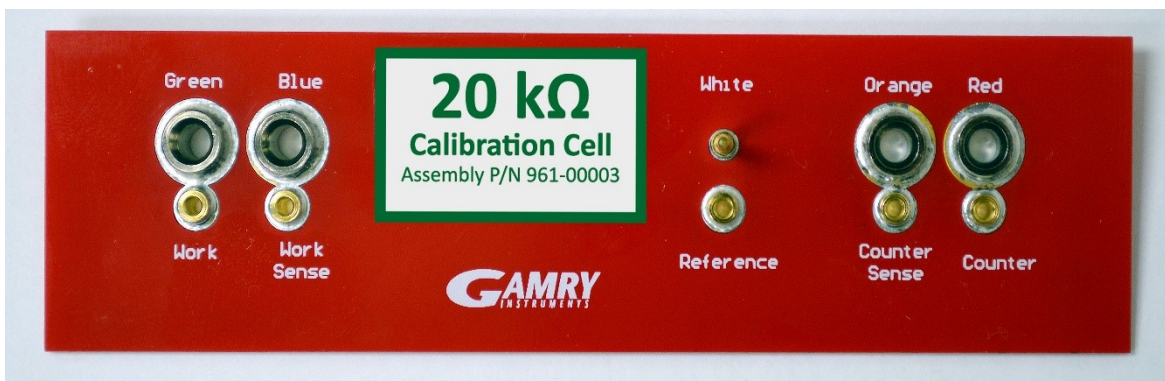
Figure 5-3 20 kΩ Calibration Cell
