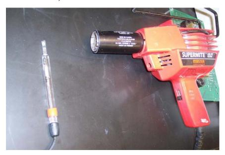
Trim the excess Teflon so that it is even with the end of the Vycor. If you do not, the excess Teflon tube can trap a gas bubble and isolate your reference electrode from the solution.
