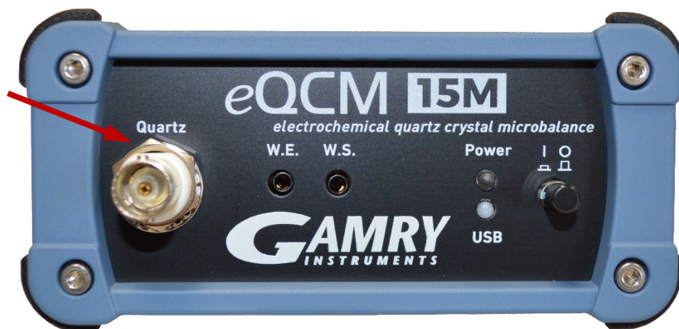
Figure 5-1 Connection of the BNC Cable to the Quartz
