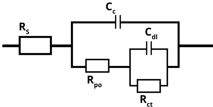
When you use EIS to test a coating, you fit a data curve to this type of model. The fit returns estimates for the model parameters, such as the pore resistance and the double layer capacitance. You then use these parameters to evaluate the degree to which the coating has failed.
