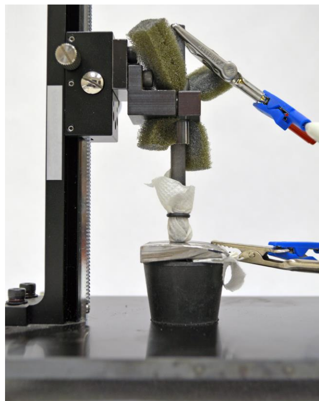
Figure 1. Overall EIS testing stage, showing curved metal sample (sitting on top of butyl-rubber stopper), with graphite rod pressing upon the sample.
