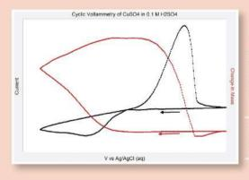
When you combine the eQCM 10M with a Gamry Potentiostat such as a Reference 600+<sup>TM</sup>, you get the combination of state-of-the-art instruments. Data are easily incorporated into Gamry's powerful Echem Analyst giving an intuitive feel to analysis and presentation. Current/Voltage curves overlaid with frequency data are standard.
