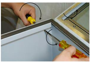
2. Place the VistaShield on top of the Stir/Purge, aligning the four screws with the four holes in the top of the Stir/Purge chassis.
