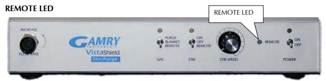
An LED is located to the left of the POWER toggle/LED. This LED is lit when one or both of the STIR or GAS switches are in the REMOTE position.
