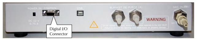
The CONTROL Digital I/O connector controls the stir and purge functions via simple digital signals from any Gamry potentiostat or other device that outputs on the proper pins.
