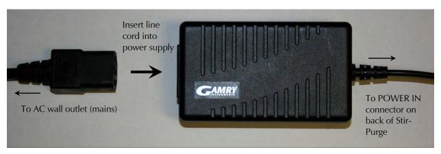
The external power supply provided with the Stir/Purge is rated for operation from 100 to 240 V AC, at frequencies from 47 to 63 Hz. It should therefore be useable worldwide.
