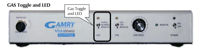
The GAS Toggle and LED are located to the left of the STIR Toggle and LED. The PURGE function of the Stir/Purge is controlled by a three-position GAS toggle switch and by the FLOW RATE knob. The three positions of the GAS toggle are (top to bottom) PURGE, BLANKET, and REMOTE:
