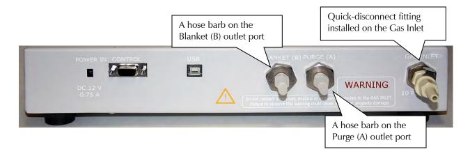
The manufacturer of the needle valve used to control gas flow rate does <u>not</u> recommend use of PTFE tape on any threaded fittings used in the inlet gas plumbing. Small pieces of the tape may escape into the gas flow and block the needle value orifice. You can use PTFE thread-seal tape on the outlet ports if you desire.
