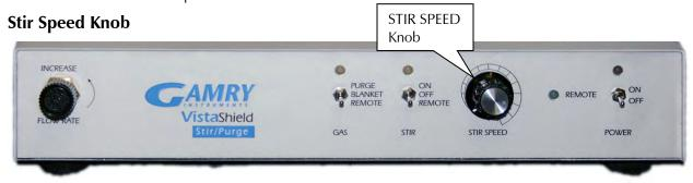
To the left of the REMOTE LED is the STIR SPEED Knob. This is a 16-position control knob. The bottom position is "Off" and the stir speed increases from the lower left, clockwise, through the remaining 15 positions
