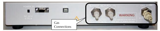
The three connections for gas flow are located on the right side of the back panel. The GAS INLET is a quick release, interchangeable hose barb on the far right, and the two gas outputs [BLANKET (B) and PURGE (A)] are case-mounted hose barbs.
