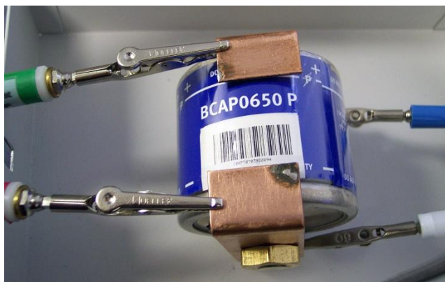
Figure 14. Connections from the potentiostat to the Maxwell capacitor.
