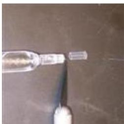
5. Refill the interior electrode body with saturated KCl. Allow the electrode to soak in saturated KCl for at least 1 hour before use to ensure the new frit is completely wet.
