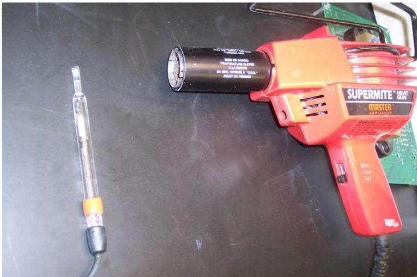
4. Trim the excess Teflon so that it is even with the end of the Vycor. If you do not, the excess Teflon tube can trap a gas bubble and isolate your reference electrode from the solution.
