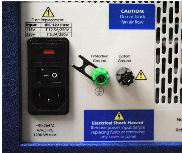
Figure B-2 Storing Ground Jumper When Disconnected
