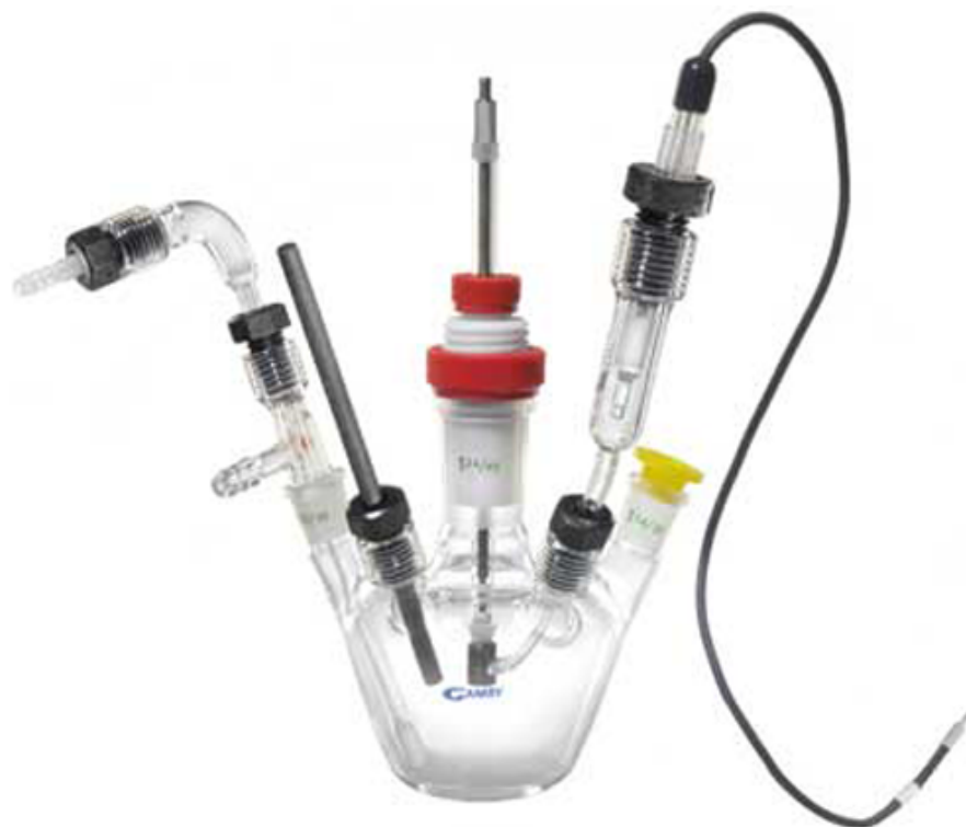
Figure 1. The Standard Configuration of a RDE Cell.
