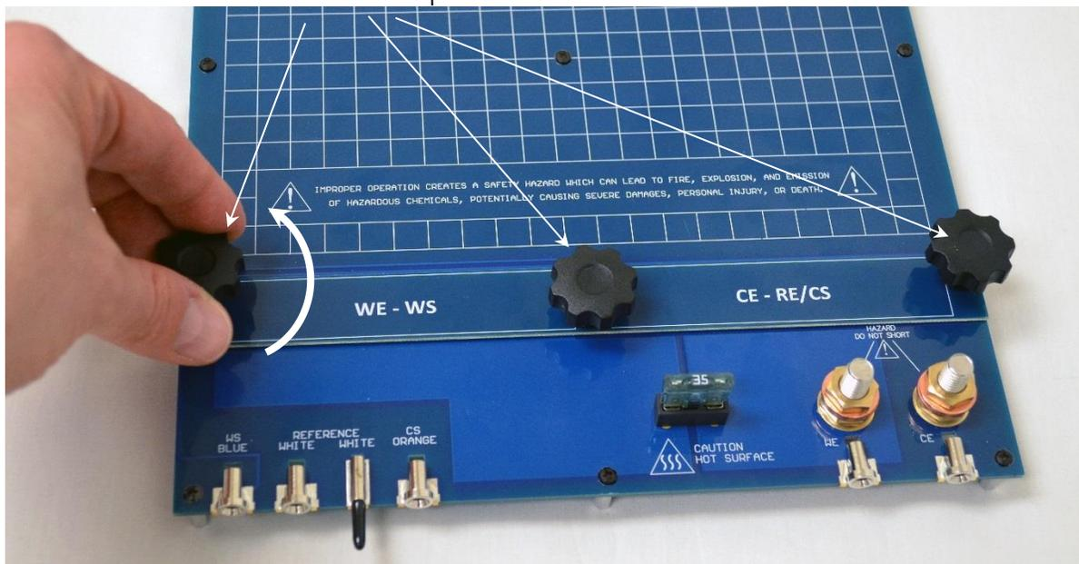
2. Carefully raise the sense clamp. (For most pouch cells you should not need to completely remove the knobs and clamp, but you may remove them if necessary.)
