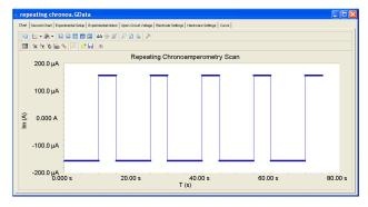
**Repeating Techniques Waveform.** This waveform is the same shape for Repeating Chronoamperometry and Repeating Chronopotentiometry. Two steps of individually specified magnitude and length are applied cyclically. Data are stored in a single file.
