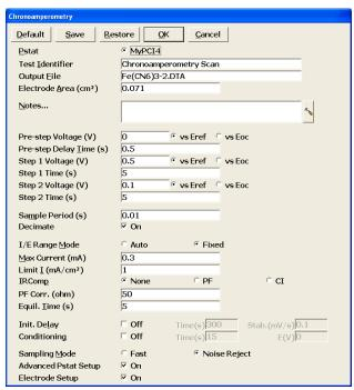
Setup Window for Chronoamperometry. Double-step chronoamperometry may be easily performed with the grant The Day WY 9 YM CWY a left of the CAR UY sets the current range based on the maximum Warent. The "Default" button resets the default values for all parameters.
