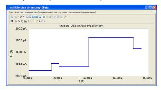
Multiple-Step Chronoamperometry Waveform. The Multi-Step experiment is for users that want to individually specify numerous steps of different sizes and durations. This is an ideal experiment to run for unique signals that do not repeat or differ by any regular increment.
