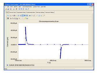
Chronoamperometry Display with Decimation. With Decimation, the rate of data acquisition decreases by a factor of ten with each decade of time. Decimation is also available in Chronocoulometry and Chronopotentiometry.
