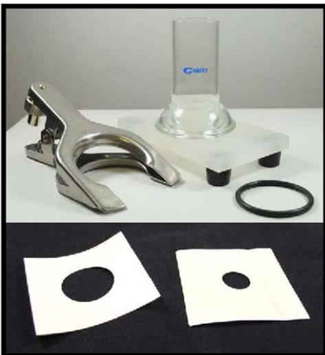
PortHoles Electrochemical Sample Masks define a known area of the sample surface for electrochemical testing with the PTC1. PortHoles are available in 1, 3, or 10 cm<sup>2</sup> area to accommodate any specimen.
