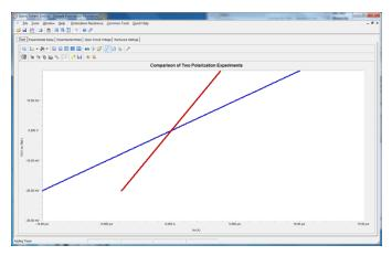
Two Polarization Resistance plots overlaid for comparison. The title has been completely changed. The **Annotation toolbar** is visible at the bottom of the display. The two plots are color-coded so they can be distinguished from each other (see the legend above the **Annotation toolbar**). The marker styles can also differentiate the traces. To calculate corrosion rate, select the portion of the curve with two mouse-clicks, then select **Polarization Resistance**.
