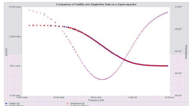
**Figure 8. The comparison of OptiEIS and a single sine spectrum for a simplified Randles dummy cell (200 Ω in series with a 2.3kΩ in parallel with 2 mF).**
