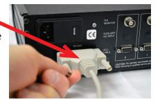
Attach the Potentiostat/ECM8 cable to the cell cable jack on your potentiostat. Attach the other end of the ECM8 cable to the multiplexer **POTENTIOSTAT** receptacle.
