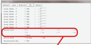
In the Active Cell area, choose a radio button for any channel to be calibrated, and click the OK button.
