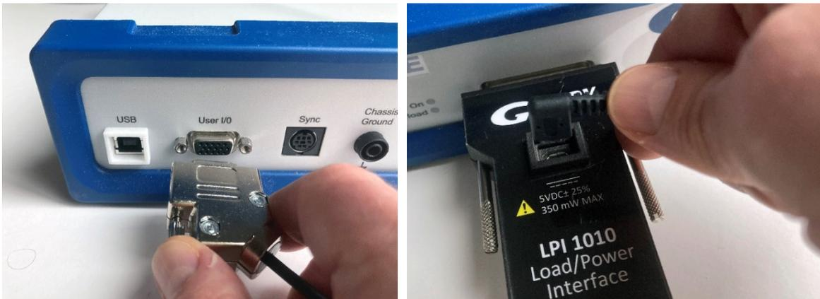
The Interface 1010 supplies a regulated 5 V output and Earth ground via the User I/O connector. Inside the LPI D-sub Module, the 5 V power is stepped up to an isolated  $\pm 15$  V power supply by way of a transformer. Thus, all circuitry connected to the cell-connector pins are isolated from Earth ground.
