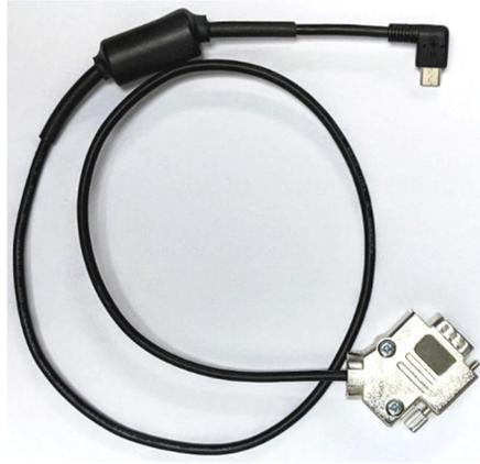
The LPI Power Cable has a 15-pin HD D-sub connector on one end which mates with the User I/O connector on the back of the Interface 1010. Hand-tighten the jackscrews on the LPI Power Cable until snug. The other end of the cable terminates in a male micro USB-B connector and plugs into the female micro USB-B connector on the top side of the LPI1010 D-sub Module as shown in Figure 4-4.
