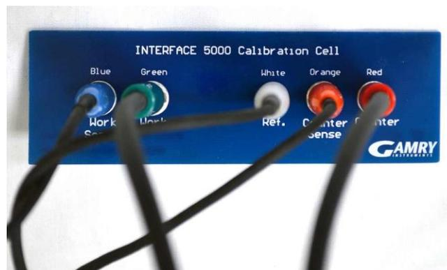
Figure 1: Calibration cell showing proper connections.
