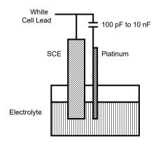
The third method involves providing a high-frequency shunt around the cell. A small capacitor between the red and white cell leads allows high-frequency feedback to bypass the cell. The capacitor's value is generally determined by trial and error. Ten nF (10 000 pF) is a good starting point.
