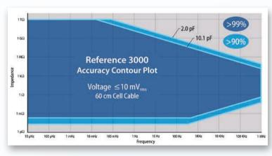
With on-board electronics for electrochemical impedance spectroscopy, the Reference 3000 can make accurate measurements over a frequency range from 10 µHz to 1 MHz. Modes include potentiostatic, galvanostatic, and a unique hybrid mode where potentiostatic EIS is run galvanostatically to ensure you don't accidentally damage your sample.
