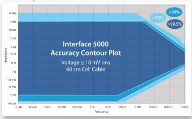
The Interface 5000 is ideal for testing low impedance devices and covers the frequency range of 10  $\mu$ Hz to 1 MHz at 99% accuracy. The current-carrying leads and sense leads have been separated to reduce mutual inductance, thereby giving you more bandwidth at low impedances. You can accurately characterize devices down to 150  $\mu\Omega$ .
