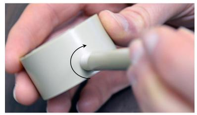
3. Seat a second O-ring (6 mm-dia.) on the green end of the cell cable.
