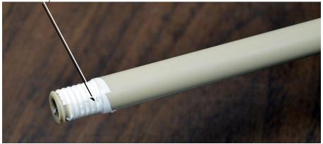
5. Screw the rod into the cell body.
