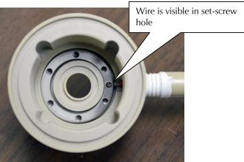
10. Thread the M2.5 set screw into its receptacle, and tighten with the small screwdriver until the top of the set screw is recessed below the metal ring.
