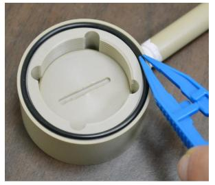
17. Screw the sealing lid onto the cell body
