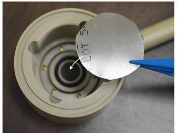
14. Drop the stopper plate into the cell body on top of your sample. Line up the tabs with the recesses in the cell body.
