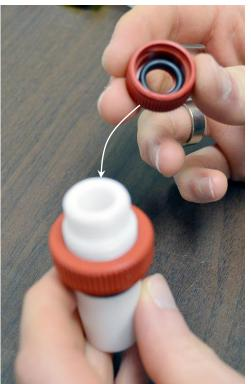
5. Insert the cell's rod through the adapter.
