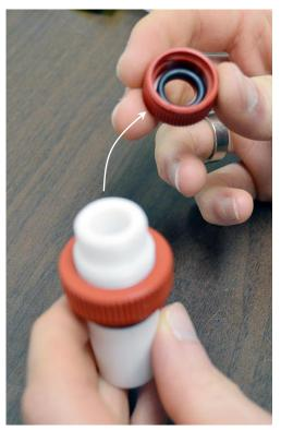
2. Remove the existing O-ring from the cap.
