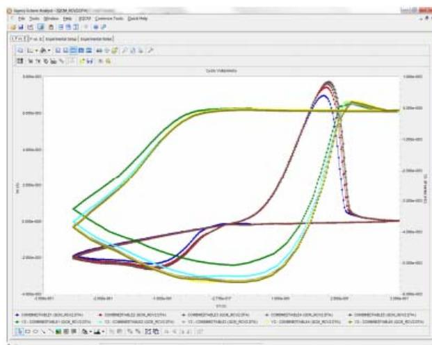
**Figure 3. Echem Analyst showing current and frequency change versus voltage for the five cycles.**
