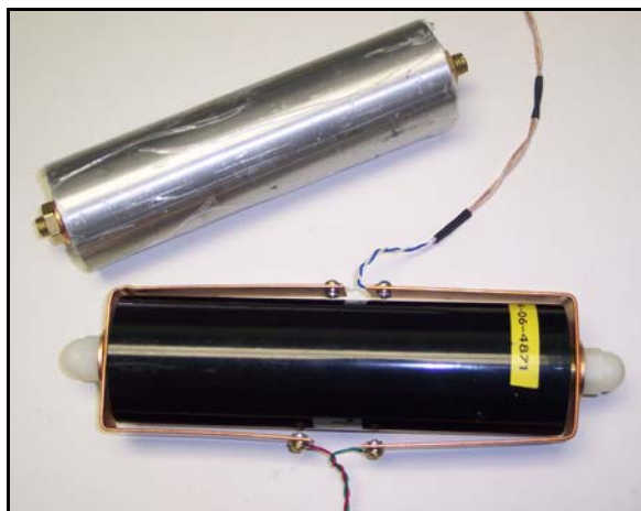
Figure 2. Battery in Fixture and Surrogate.
