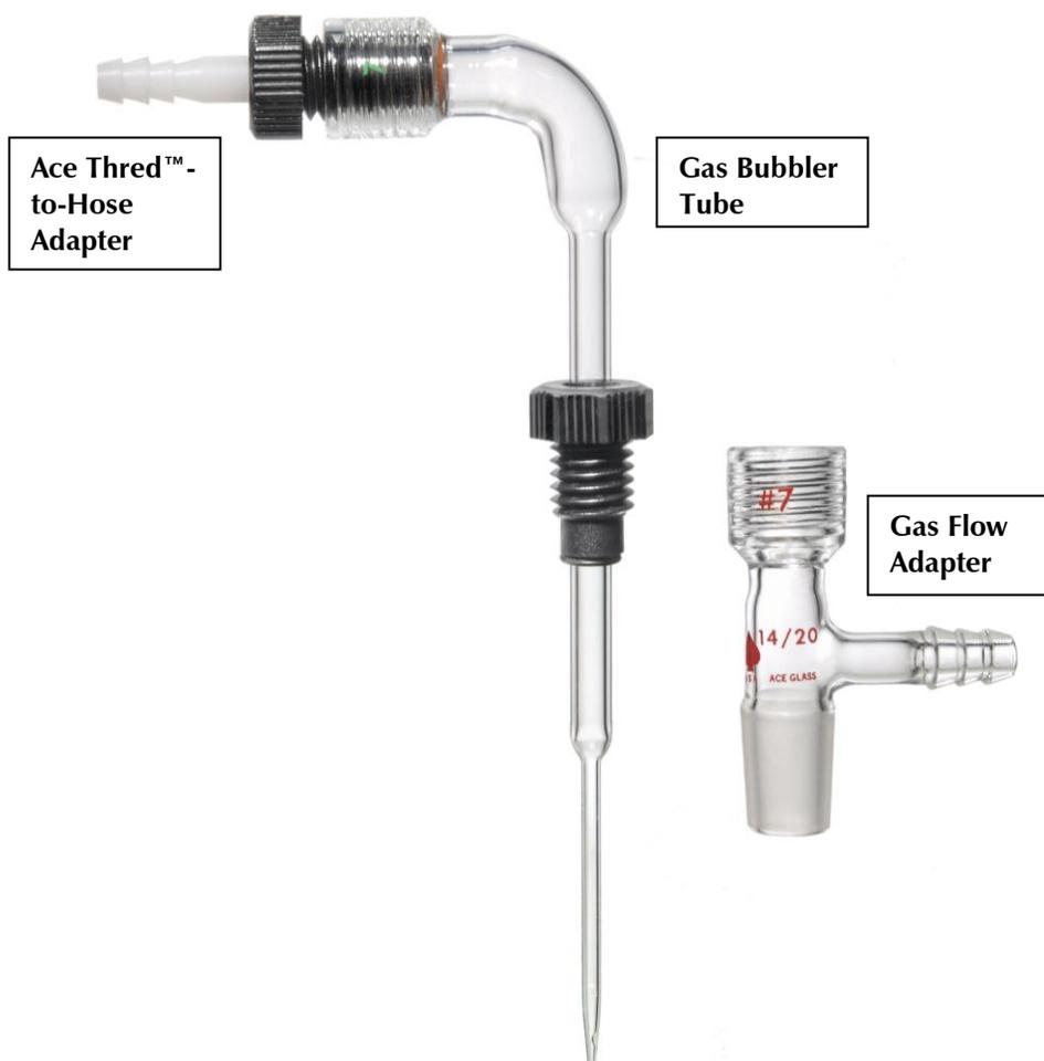
Figure 3 is representative of the Gas Bubbler used for purge only (no blanketing). Connect one end of a plastic hose (not shown) to the Gas Bubbler Tube using the ACE-Thred™-To-Hose adapter. Connect the other end of this hose to a source of purge gas.
