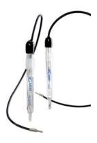
The impedance of your Reference Electrode should be less than 1 kohm. An impedance higher than 1 kohm is not good and an impedance higher than 5 kohm is unacceptable and must be corrected. With a Gamry Reference Electrode, the problem is easily corrected by changing the Porous Glass Frit.
