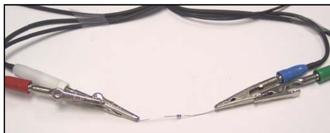
Figure 5 – Preferred orientation for alligator clips to minimize the capacitive contribution from the clips (optimized plate area).
