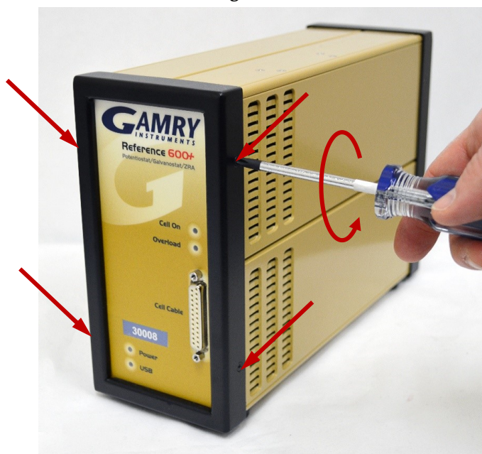
Figure 4-5 Removing the Front Bezel
