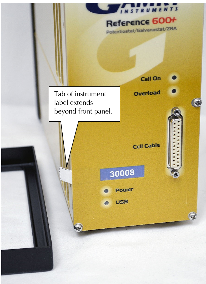
Figure 4-6 Removing the Front Bezel
