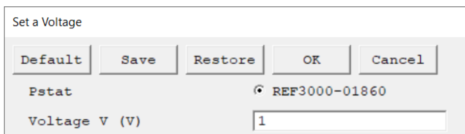
Figure 6-3 Setup Dialog Box for the "Set a Voltage" Script
