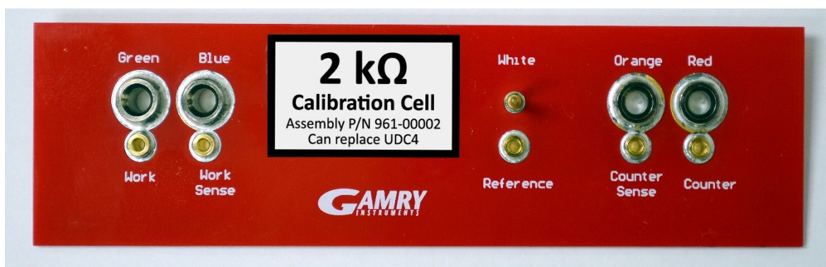
Figure 5-1 2 k \Omega Calibration Cell
