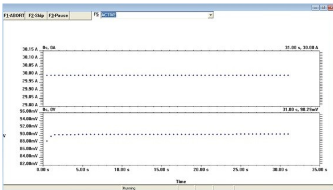
Figure 6-4 Typical Runner Window with Good Fuses
