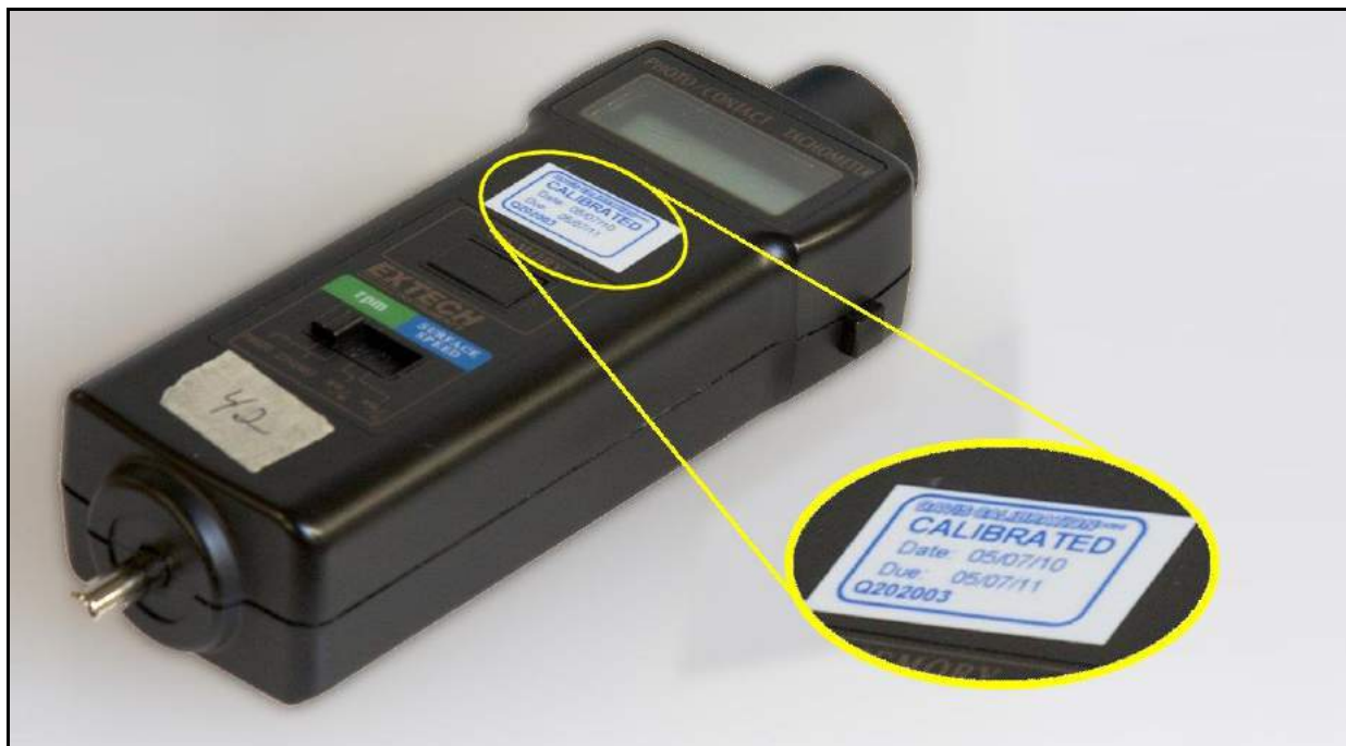
Figure 6.1: An Optical Tachometer with a Traceable Calibration Certificate
