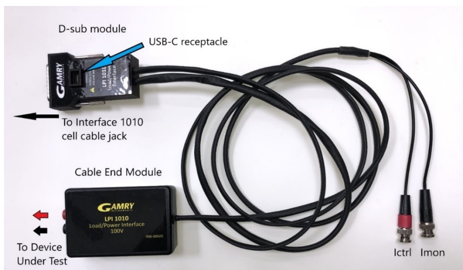
Figure 3-1 Overview of the LPI1010 Top-Level Assembly
