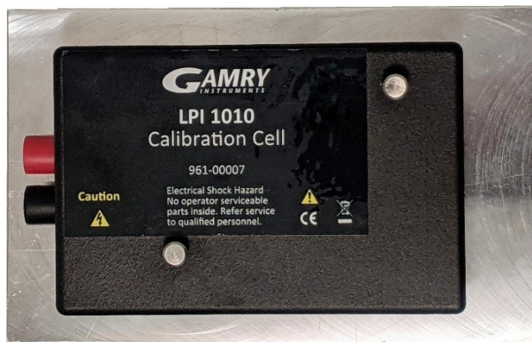
Figure 5-3 LPI1010 200 m \Omega Calibration Cell with cover
