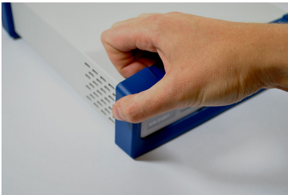
Figure 3-4 Removing the Front Bezel
