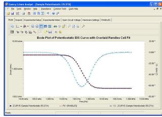
**A** Bode Plot of a Randles Cell with the fit overlaid on the data. Click the "Randles" tab to view the values of the elements in the equivalent circuit and the Goodness of Fit coefficient.
