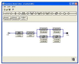
**The EIS300 Model Editor** employs an easy-to-use click-and-drag mechanism to build an equivalent circuit. Build it once and save it.
