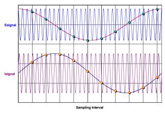
**Sub-Harmonic Sampling** transforms the high-frequency voltage and current signals to a lower frequency while maintaining the amplitude and the phase relationship.
