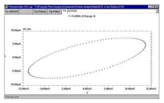
A Lissajous Figure Displayed During Data Acquisition provides a snapshot of the data quality and potentiostat performance.
