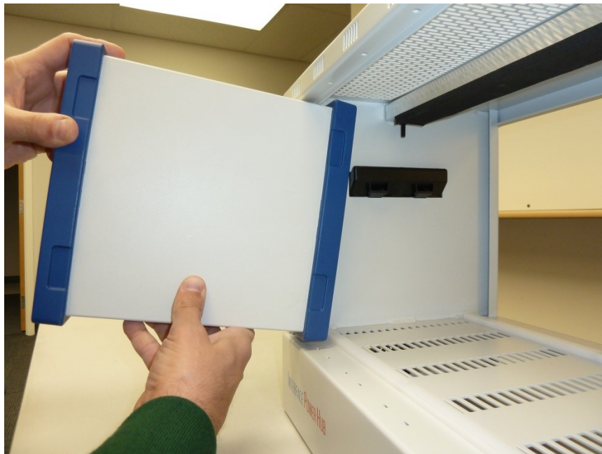
Figure 3-6 Tilting the Instrument to Place it in the IPH Chassis
