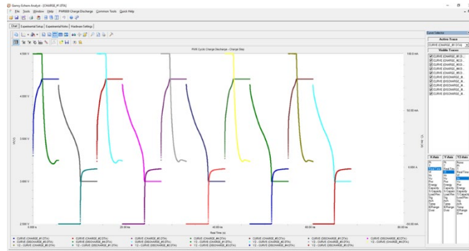
Figure 7- IV plot of the charge and discharge cycles plotted against time. The Show Curve Selector button is selected in the top left of the screen
