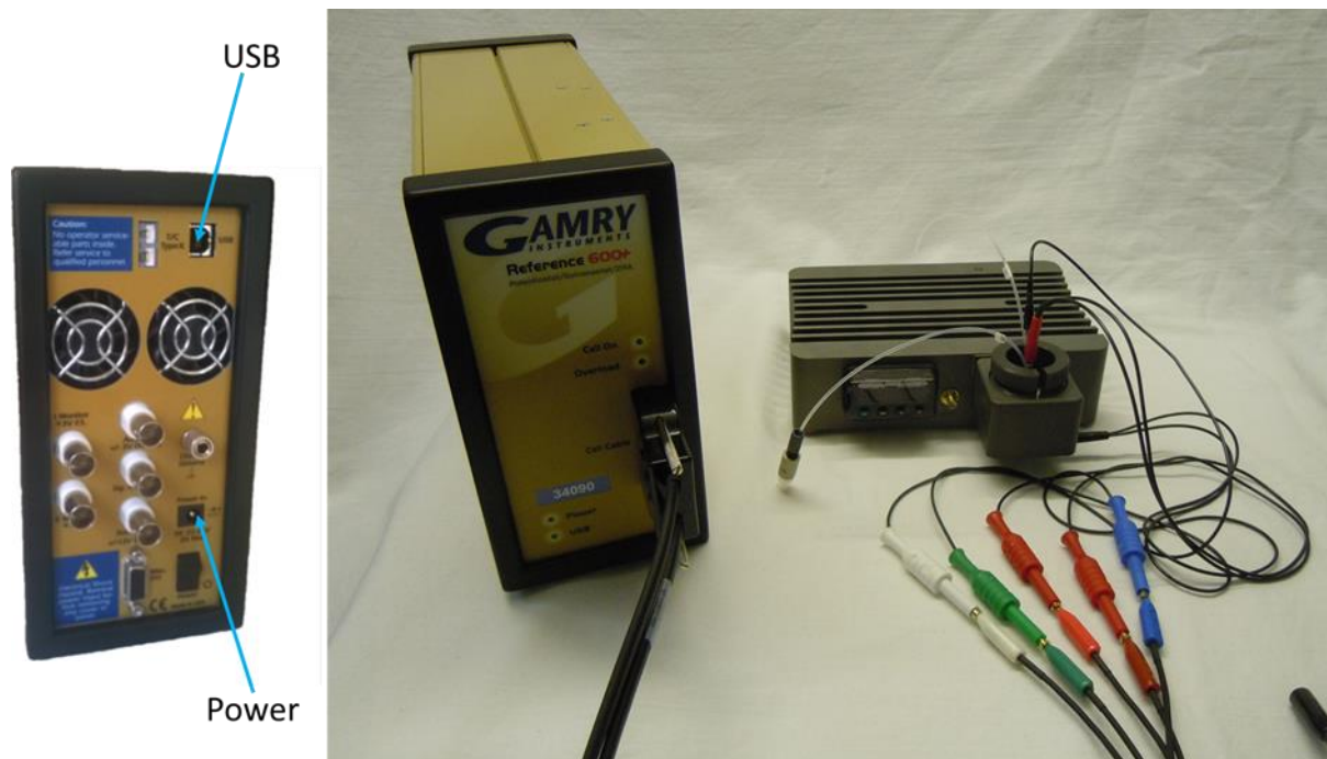
Figure 2: Gamry Potentiostat and QCM-I Mini, showing the Reference (white), counter (red), counter sense (orange) and working electrode (green) and working sense (blue) connections.
