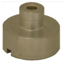
Figure 34: 5 MHz Dummy Sensor Module with alignment notch for Channel A thermal chamber.
