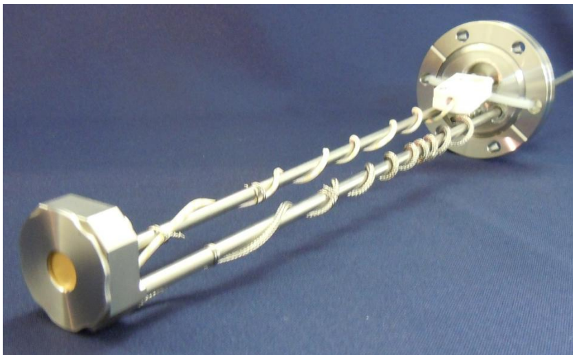
Figure 23: QCM sensor holder for vacuum application with CF feedthrough and temperature measurement.
