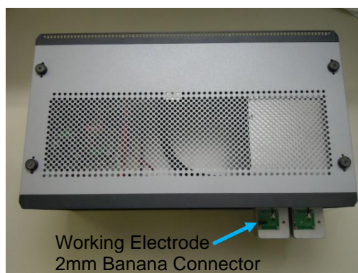
Figure 5: QCM-I measurement unit's underside view showing EC working electrode connector.
