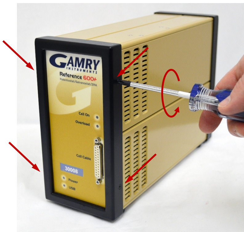
Figure 4-5 Removing the Front Bezel
