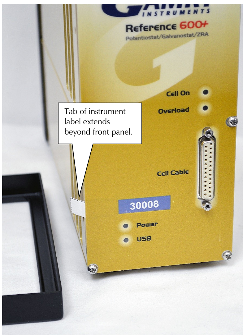
Figure 4-6 Removing the Front Bezel
