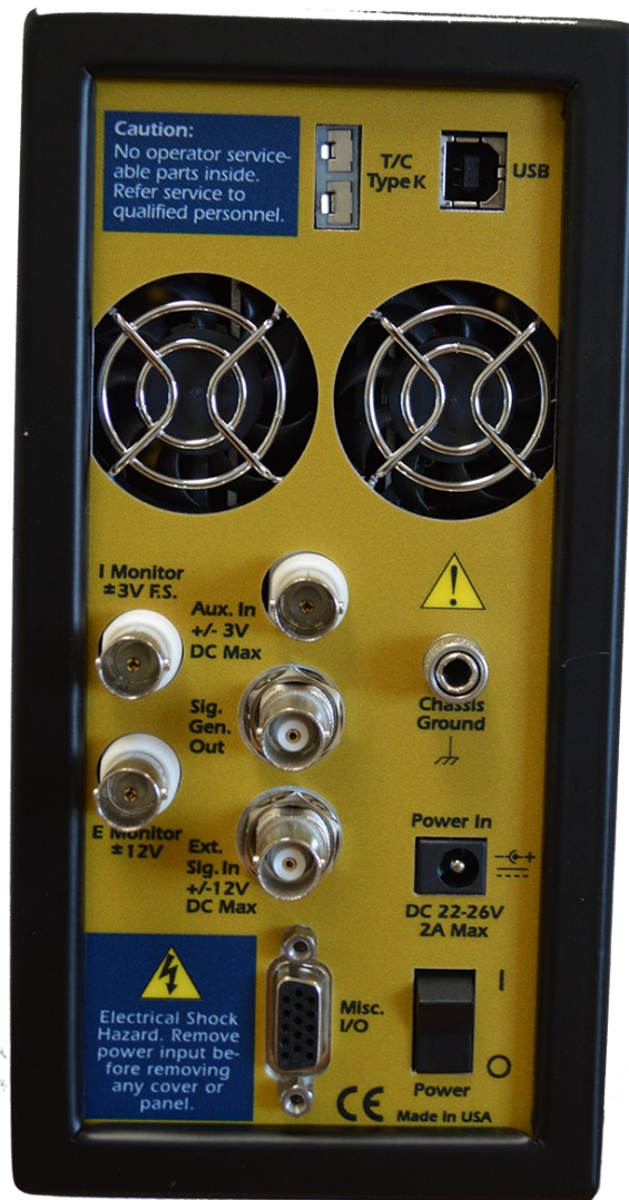
Figure 4-2 Rear Panel of the Reference 620
