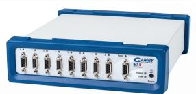
The IMX8 partners with a Gamry Instruments potentiostat to convert a single potentiostat into a powerful instrument suitable for sequential multichannel operations. Each multiplexer allows you to sequentially take measurements on up to eight electrochemical cells. The IMX8 is great for automating repetitive experiments, and for increasing throughput on long-term experiments where data can be taken periodically.
