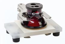
The design of the PTC1 Paint Test Cell is very simple in order to keep cost down, for most users require many cells for testing. The flat sample under test is clamped between a glass tube with an O-ring seal and the PTFE base. The tube is partly filled (20–50 mL) with the test electrolyte and sealed with a rubber stopper. A reference electrode (possibly saturated calomel) and a graphite rod counter electrode are mounted through the stopper.
