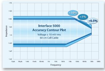
The Interface 5000 is ideal for testing low impedance devices and covers the frequency range of 10  $\mu$ Hz to 1 MHz at 99% accuracy. The current-carrying leads and sense leads have been separated to reduce mutual inductance, thereby giving you more bandwidth at low impedances. You can accurately characterize devices down to 150  $\mu\Omega$ .
