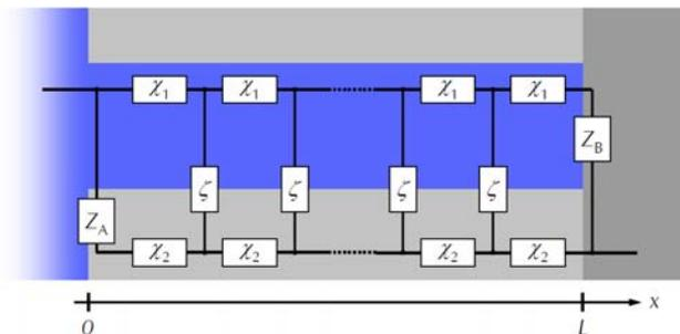
Figure 3 – Scheme of a generic transmission line model.
