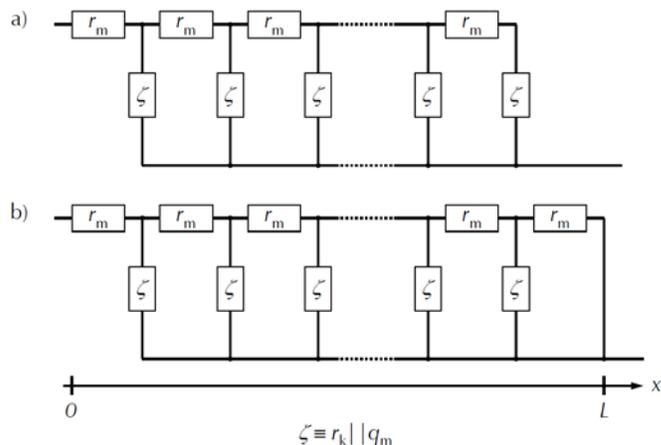
**Figure 5** – Two specific cases of transmission line models. (a) Bisquet Open (BTO) and (b) Bisquet Short (BTS). For details, see text.
