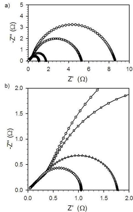
**Figure 10** – a) Simulated data for the circuit depicted in Figure 9 with different reaction resistances  $R_B$ . b) Segment of the spectra. ( $\diamond$ )  $R_B = 0.1 \Omega$ , ( $\triangle$ )  $R_B = 1 \Omega$ , ( $\square$ )  $R_B = 10 \Omega$ , ( $\circ$ )  $R_B = 100 \Omega$ . For details, see text.
