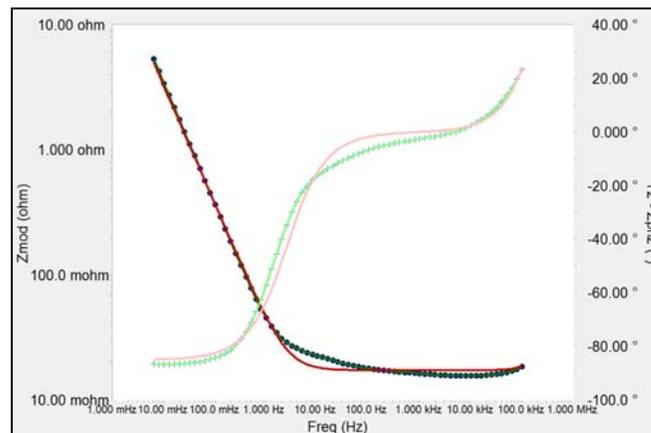
**Figure 6** – Bode diagram of a potentiostatic EIS test on a 5 F EDLC (●). (●) R-CPE model, (●) modified "Bisquert Open" model. (●) magnitude, (+) phase. For details, see text.
