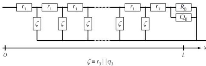
**Figure 9** – Scheme of a transmission line model to describe TiO<sub>2</sub>/organic hole conductor DSCs. For details, see text.
