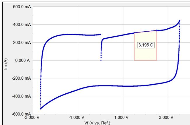
**Figure 5** – CV curve of a 3 F EDLC. Current versus voltage are shown for the first cycle. For details, see text.
