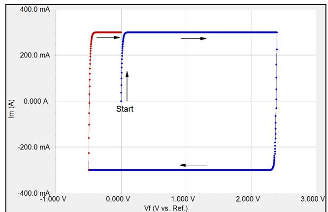
**Figure 4** – Theoretical CV curve of a 3 F EDLC. Current versus voltage are shown for the first two cycles. For details, see text.
