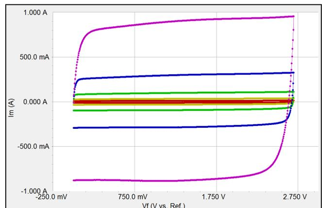
**Figure 6** – CV curves of a 3 F EDLC with varying scan rates.
