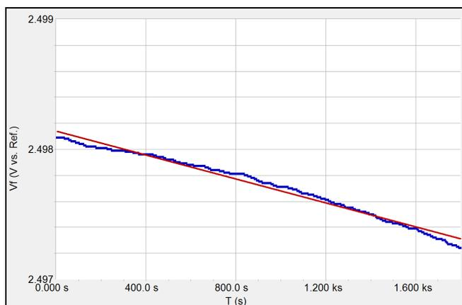
**Figure 11** – Self-discharge measurement on a 3 F EDLC.
