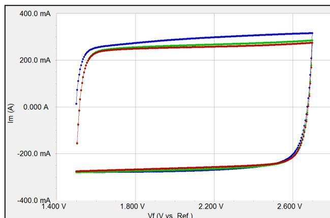
**Figure 8** – Different cycles of a CV test of a 3 F EDLC. (●) 1<sup>st</sup> cycle, (●) 10<sup>th</sup> cycle, (●) 50<sup>th</sup> cycle. For details, see text.
