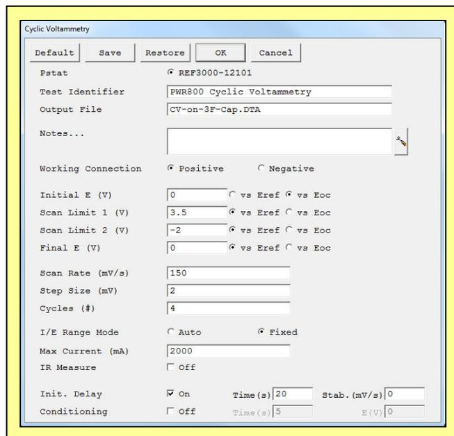
**Figure 3** – Gamry's PWR800 setup for a CV experiment.
