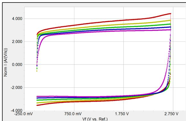
**Figure 7** – Scan rate normalized CV curves of a 3 F EDLC with varying scan rates. (●) 316 mV/s, (●) 100 mV/s, (●) 31.6 mV/s, (●) 10 mV/s, (●) 3.16 mV/s. For details, see text.
