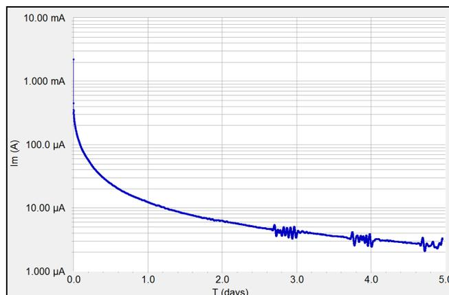
**Figure 10** – Leakage current measurement on a 3 F EDLC over five days at 2.5 V. For details, see text.
