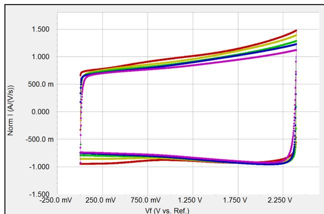
**Figure 9** – Scan rate normalized CV curves of a 1 F PAS pseudocapacitor with varying scan rates. (●) 316 mV/s, (●) 100 mV/s, (●) 31.6 mV/s, (●) 10 mV/s, (●) 3.16 mV/s. For details, see text.
