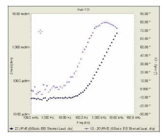
This spectrum fits well to a series RL model with a resistance of 30  $\mu\Omega$  and inductance of 42 nH. The resistance value is interesting. The copper braid used to make the shorted connection has a measured resistance of 8.4  $\mu\Omega$  per mm. 30  $\mu\Omega$  corresponds to a path of 3.6 mm through the braid.
