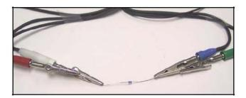
Record the potentiostatic EIS spectrum of this resistor with zero DC and 20 mVrms AC voltage. The frequency range should extend from 0.2 Hz to the system's maximum specified frequency.
