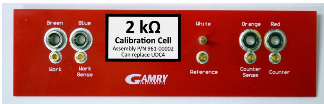
Figure 4-1 2 k \Omega Calibration Cell
