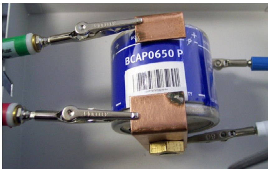
Figure 39. Electrode connections for measurements on a 650 F EDLC. Working (green), Counter (red), Working sense (blue), and Reference (white).
