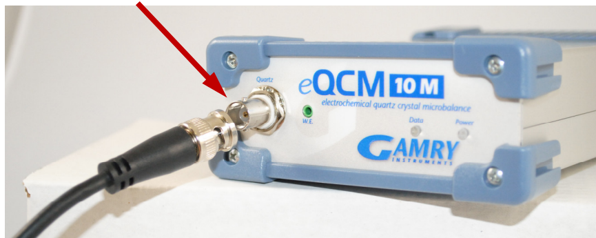
Figure 5-1 Connection of the Cell Cable
