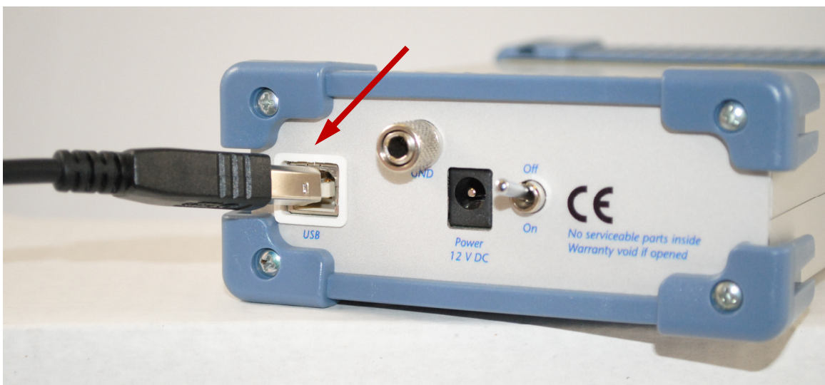
Figure 4-3 Rear panel of the eQCM 10M with USB cable
