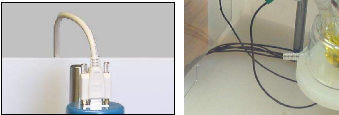
Figure 4.10: Routing Cables out of the Enclosure
