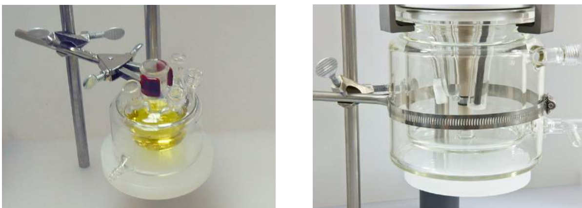
Figure 4.5: Properly Supported and Clamped Electrochemical Cells
