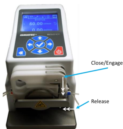
Figure2: Peristaltic pump, 12 roller, 2 channel ICC.
