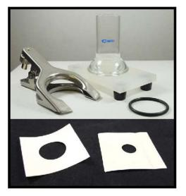
PortHoles Electrochemical Sample Masks define a kown area of the sample surface for electrochemical testing with the PTC1. PortHoles are available in 1, 3, or 10 cm<sup>2</sup> area to accommodate any specimen.
